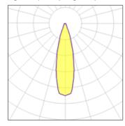
LED CCT 2700 K Lamp type Nominal lamp power 6 W CRI 80 Total flux LOR 100% 515 lm Luminous efficacy 86 lm/W Total power 6 W
