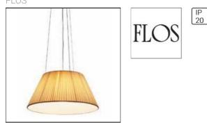
Suspension fixture providing diffused lighting. Acid-etched pressed borosilicate glass internal diffuser. Plissé cloth shade. Injection-molded transparent polycarbo-nate diffuser support.Transparent, stamped polycarbonate dust protection screen.White, injection-molded ABS rose, galva-nized pressed steel ceiling fitting. Steel suspension cables and polarized double-insulated PTFE cord, length 4000 mm.Net weight 3,4 kg.
