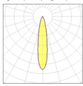
CCT Lamp type LED 3000 K Nominal lamp power 2.75 W CRI 90 Total flux 198 lm LOR 100% Luminous efficacy 72 lm/W Total power 2.75 W
