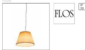
Suspension fixture providing diffused lighting. Acid-etched pressed borosilicate glass internal diffuser.Plissé cloth shade. Injection-molded tran-sparent polycarbonate diffuser support. Transparent, stamped polycarbonate dust protection screen. White, injection-molded ABS rose, galva-nized pressed steel ceiling fitting. Steel suspension cables and polarized double-insulated PTFE cord, length 4000 mm.Net weight 1,6 kg.
