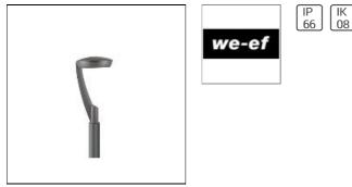
IP66, Class I. Marine-grade die-cast aluminium alloy. 5CE superior corrosion protection including PCS hardware. Silicone rubber gaskets. Safety glass lens. Control gear on hinged and 'no tool' removable gear tray. Anodised aluminium reflector, for beam efficiency and glare control. 'No tool' lamp replacement. Recommended mounting height 2,5-8,0 m, depending on lamp type selected.
