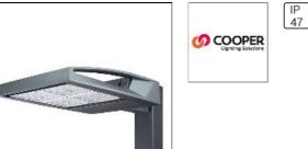
Choice of 16 high-efficiency, patented AccuLED Optics™, 3,400 - 61,800 lumens, up to 131 lp/W, Standard in 4000K CCT, 70 CRI, optional 2700K, 3000K, 5000K and 6000K, -40°C to 40°C operating range, 120-277V 50/60Hz, 347V 60Hz or 480V 60Hz operation, IP66 rated housing and LED Light Squares, Thermally conductive polymer heatsink for up to 22% weight reduction, Pole, mast-arm or wall-mounted configurations, 3G vibration rated, Five-year warranty
