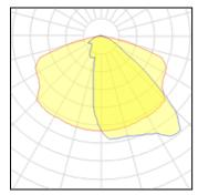
1 x LED Nominal lamp power 72 W LOR 73% Lamp flux 8460 lm Total flux 6143 lm Luminous efficacy 118 lm/W Total power 80 W CCT 3000 K CRI 80
