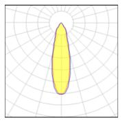
4000 K Lamp type LED CCT Nominal lamp power 2.62 W CRI 90 Total flux 218 lm LOR 100% Luminous efficacy 83 lm/W Total power 2.62 W
