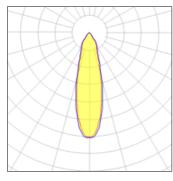
CCT 4000 K Lamp type LED Nominal lamp power 2.62 W CRI 90 Total flux 218 lm LOR 100% Luminous efficacy 83 lm/W Total power 2.62 W
