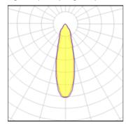
LED CCT 4000 K Lamp type Nominal lamp power 2.62 W CRI 90 Total flux 218 lm LOR 100% 83 lm/W 2.62 W Luminous efficacy Total power
