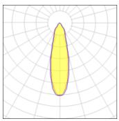
CCT Lamp type LED 4000 K Nominal lamp power 2.62 W CRI 90 Total flux 218 lm LOR 100% Luminous efficacy 83 lm/W Total power 2.62 W
