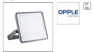
Housing: Die-cast Aluminum; Mounting ring: Grey; Installation: Bracket/ Pole; Dimensions: 352\*363\*54mm; Ceiling cutouts: /; Beam angle: 35°\*80°; Lamp(s): LED; Power: 200W; Efficacy : 95Lm/w Total luminous flux of luminaire: 20000lm; Power Factor: 0.95 Mains voltage: AC220-240V/50-60Hz; Colour temperature: 5700K; Colour rendering: Ra80; UGR: / IP/IK Grade: IP66/ IK06; Class of protection I; Control System: / Service life: 30,000h at 70% luminous flux;
