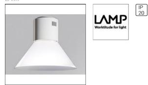
Suspended downlight model STORMBELL 3000 WW FL WH/WH., LAMP brand. Made of shiny white extruded and injected aluminum body with polycarbonate opal ring. Model for COB with warm white color temperature and control gear included on white decorative rose. Flood aluminum reflector. Insulation class I.
