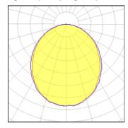
LED CCT 4032 K Lamp type Nominal lamp power 28.75 W CRI 80 Total flux 3438 lm LOR 100% 120 lm/W 28.75 W Luminous efficacy Total power
