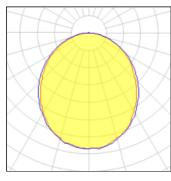
CCT 4032 K Lamp type LED Nominal lamp power 28.75 W CRI 80 Total flux 3438 lm LOR 100% Luminous efficacy 120 lm/W Total power 28.75 W
