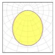
4032 K Lamp type LED CCT Nominal lamp power 28.75 W CRI 80 Total flux 3438 lm LOR 100% Luminous efficacy 120 lm/W 28.75 W Total power
