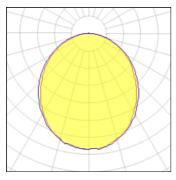
Lamp type LED CCT 4032 K Nominal lamp power 28.75 W CRI 80 Total flux 3438 lm LOR 100% Luminous efficacy 120 lm/W Total power 28.75 W
