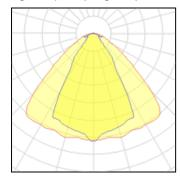
Lamp typeLEDCCTNominal lamp power25 WCRITotal flux1050 lmLORLuminous efficacy42 lm/WTotal power
