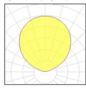
LED CCT 2665 K Lamp type Nominal lamp power 1 W CRI 80 Total flux 100% 10 lm LOR Luminous efficacy 10 lm/W ULOR 100% Total power 1 W
