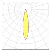
1 x LED LOR 73% Nominal lamp power 6 W Lamp flux 945 lm Total flux 687 lm Luminous efficacy 158 lm/W Total power 6 W ССТ 3000 K CRI 90
