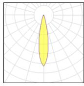
1 x LED Nominal lamp power LOR 73% 6 W 687 lm Lamp flux 945 lm Total flux 158 lm/W Total power 6 W Luminous efficacy CCT 3000 K CRI 90
