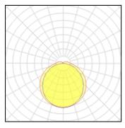
Lamp type LED CCT 3000 K Nominal lamp power 16 W CRI 80 Total flux 1869 lm LOR 100% Luminous efficacy 117 lm/W ULOR 7% Total power 16 W
