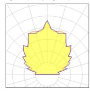
Lamp type LED CCT 3000 K Nominal lamp power 1 W CRI 80 Total flux LOR 100% 56 lm Luminous efficacy 56 lm/W ULOR 98% Total power 1 W
