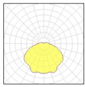
CCT 2700 K Lamp type LED Nominal lamp power 96 W CRI 90 LOR 100% Total flux 4684 lm Luminous efficacy 49 lm/W ULOR 10% Total power 96 W
