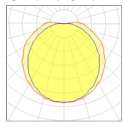
LED CCT 4000 K Lamp type Nominal lamp power 50 W CRI 80 Total flux LOR 100% 8000 lm Luminous efficacy 160 lm/W ULOR 3% Total power 50 W
