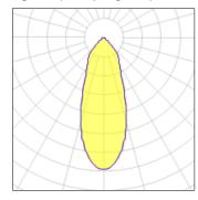
Lamp type LED CCT 3000 K Nominal lamp power 7.5 W CRI 80 Total flux LOR 100% 430 lm Luminous efficacy 57 lm/W Total power 7.5 W
