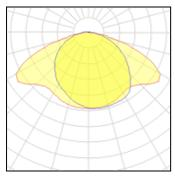
1 x Metal halide lampNominal lamp power150 WLamp flux15000 lmLuminous efficacy69 lm/WCCT2900 KCRI90
