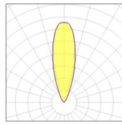
LED CCT 4000 K Lamp type Nominal lamp power 1.9 W CRI 80 Total flux 77 Im LOR 100% Luminous efficacy 41 lm/W ULOR 100% Total power 1.9 W
