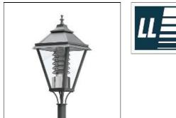
recom. pole height: 3.00m - 5.00m light standards: low and medium lighting requirements lamp: incl. 1 glare-free U LED module colour temperature: 3.000K warm white or 4.000K neutral white LED gear: electronic driver, up to 85.000 hours, high efficiency factor of 94%, with soft start function and Constant Light Output (CLO) in order to keep the luminous flux the same over the entire life time LED life expectancy: up
