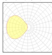
Lamp type LED CCT 4000 K Nominal lamp power 6.7 W CRI 82 Total flux 1077 lm LOR 100% Luminous efficacy 161 lm/W ULOR 50% Total power 6.7 W
