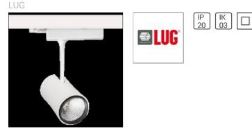
The luminaire dedicated for commercial space lighting (HI-CRI), but also, with usage of adequate LED source (FOOD technology), for product exhibition places, additional special lighting Boutiques, True Color. Mounting: in 3-phase track Body: high pressure die-cast aluminum Power: 220-240V 50/60Hz Lifetime (L80B10): 40 000 h Operating temperature range: 0°C ... +35°C Warranty: 5 years Application: boutiques, delicatessen, jeweler, shopping centers, supermarkets, museums
