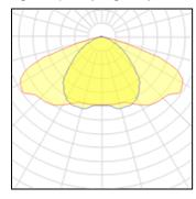
Lamp type Nominal lamp power Total flux Luminous efficacy LED 67 W 7280 lm 109 lm/W CCT CRI LOR Total power 4000 K 80 100%
