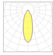
1 x LED Nominal lamp power 22 W Lamp flux 1750 lm Luminous efficacy 77 lm/W 3000 K CRI
