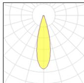
1 x LED Nominal lamp power LOR 100% 4.19 W Total flux Lamp flux 310 lm 310 lm Luminous efficacy 74 lm/W Total power 4.19 W CCT 4000 K CRI 90
