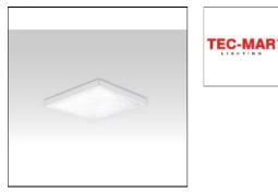
Multi-installation LED fitting, suitable for recessed installation in false ceiling with visible structure 15/24mm, surface mounting or suspended (suspension kit needed). Steel sheet body, painted with embossed white anti-yellowing epoxypolyester powder, including phosphating and degreasing pre-treatment. Electronic driver 220-240V 50/60 Hz. Manufactured in accordance with EN / IEC 60598-1.
