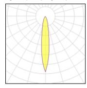
LED CCT 2700 K Lamp type Nominal lamp power 7.3 W CRI 90 Total flux LOR 100% 644 lm Luminous efficacy 88 lm/W Total power 7.3 W
