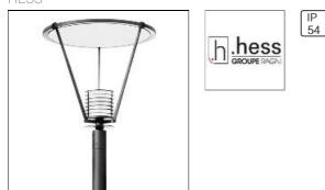
Round luminaire canopy made of thick-walled aluminium, painted white on the inside, illuminated from below. Support elements made of cast aluminium. Cylindrical luminaire glass made of borosilicate glass, top closed with single-pane tempered safety glass, framed by aluminium louvres. Luminaire body made of aluminium. Hess quality pole, cylindrically stepped, steel, galvanised, optionally with continuous embedded base or flange plate
