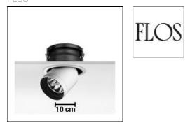
Recessed luminaire for indoor application. For very low voltage halogen lamps or standard and discharge lamps. Self-extinguishing ceramic or engineering plastic lamp holders, with single-pole, transparent electric wires with double Teflon insulation.
