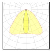
1 x LED Nominal lamp power 72 W LOR 82% Lamp flux 8460 lm Total flux 6933 lm Luminous efficacy 118 lm/W Total power 80 W CCT 3000 K CRI 80
