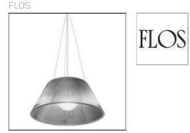
Suspension fixture providing diffused lighting. Acid-etched pressed borosilicate glass internal diffuser. Pressed clear glass shade. Injectionmolded transparent poly-carbonate diffuser support. Transparent, stamped polycarbonate dust protection screen. White, injection-molded ABS rose, galva-nized pressed steel ceiling fitting. Steel suspension cables, and polarized double-insulated PTFE cord, length 4000 mm.Net weight 7,6 kg.
