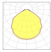
Lamp typeLEDCCTNominal lamp power6 WCRITotal flux586 lmLORLuminous efficacy98 lm/WTotal power
