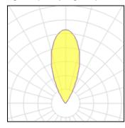
LED CCT 2665 K Lamp type Nominal lamp power 2.9 W CRI 80 Total flux 100% 279 lm LOR Luminous efficacy 96 lm/W ULOR 100% Total power 2.9 W
