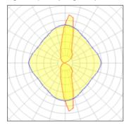
LED CCT 3000 K Lamp type Nominal lamp power 2.3 W CRI Total flux 10 lm LOR 100% Luminous efficacy 4 lm/W ULOR 50% Total power 2.3 W
