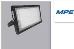
Led flood light - Lamp body made of powder coated aluminum - Lighting surface is protected by tempered glass - Ingress Protection IP65 - Driver is integrated inside the lamp - Size: 400 x 350 x 53.5 mm - Voltage: 100-240VAC - Power: 200W - Power Factor (PF): >0.95 - Luminance:
