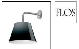
Wall or floor luminaires for outdoor use providing direct and diffused light. The outdoor range of luminaires has: a die-cast aluminum alloy wall or ceiling fitting with brillant finish; an injection-molded polycarbonate (PC) cover rose; a 316L stainless steel stem-polished; an opal-colored, vacuum-formed internal polycarbonate diffuser
