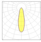
CCT 2700 K Lamp type LED Nominal lamp power 2.81 W CRI 90 Total flux 191 lm LOR 100% Luminous efficacy 68 lm/W Total power 2.81 W
