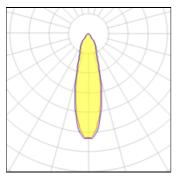
2700 K Lamp type LED CCT Nominal lamp power 2.81 W CRI 90 Total flux 191 lm LOR 100% Luminous efficacy 68 lm/W Total power 2.81 W
