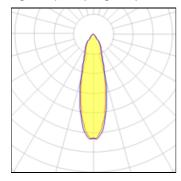
LED CCT 2700 K Lamp type Nominal lamp power 2.81 W CRI 90 Total flux 191 lm LOR 100% 68 lm/W Luminous efficacy Total power 2.81 W
