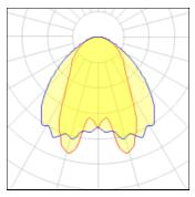
Lamp typeLEDNominal lamp power48 WTotal flux6800 lmLuminous efficacy142 lm/W
