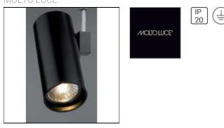
Shooter 1, Cylindrical Track Spotlight with 2-phase Volare Diretta- adapter, its simple and compact design is ideal for accent lighting; made of high-quality, die-cast aluminum; white powder coated finish; lamp replace without tools by "Slide Change"; adapter white; 1x max.50W QPAR16 GU10, 230V; 340 ° rotation and 90 ° tilt, IP 20;
