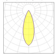
LED CCT 3000 K Lamp type Nominal lamp power 11 W CRI 80 Total flux LOR 100% 364 lm Luminous efficacy 33 lm/W Total power 11 W
