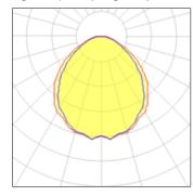
LED CCT 3000 K Lamp type Nominal lamp power 20 W CRI 80 Total flux LOR 100% 993 lm Luminous efficacy 50 lm/W Total power 20 W
