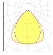
Lamp type LED CCT 4000 K Nominal lamp power 28 W CRI 80 Total flux LOR 100% 3450 lm Luminous efficacy 123 lm/W Total power 28 W
