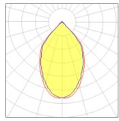
Lamp type LED CCT 3000 K Nominal lamp power 27 W CRI 80 Total flux LOR 100% 2450 lm Luminous efficacy 91 lm/W Total power 27 W
