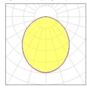
Lamp type Nominal lamp power Total flux Luminous efficacy LED 12 W 1000 lm 83 lm/W CCT
