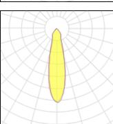
CRI 90 1 x LED Nominal lamp power 23.6 W LOR Lamp flux 1943 lm Total flux 1795 lm Luminous efficacy 76 lm/W Total power 23.6 W 2700 K CCT CRI 90 1 x LED Nominal lamp power 16.25 W LOR Lamp flux 1461 lm Total flux 1350 lm Luminous efficacy 83 lm/W Total power 16.25 W CCT 2700 K CRI 90
