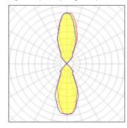
Lamp type LED CCT 3000 K Nominal lamp power 19.5 W CRI 80 Total flux 1000 lm LOR 100% Luminous efficacy 51 lm/W ULOR 46% Total power 19.5 W
