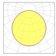
Lamp type Nominal lamp power 66 W Total flux 5683 lm Luminous efficacy 86 lm/W
