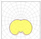
1 x Metal halide lamp Nominal lamp power 35 W Socket G12 Lamp flux LOR 3300 lm 9% Luminous efficacy 6 lm/W Total flux 285 lm CCT 4000 K Total power 48 W CRI 98
