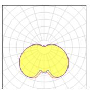
1 x Metal halide lamp Nominal lamp power 35 W Socket G12 Lamp flux 3300 lm LOR 9% Luminous efficacy 6 lm/W Total flux 285 lm CCT 3000 K Total power 48 W CRI 84
